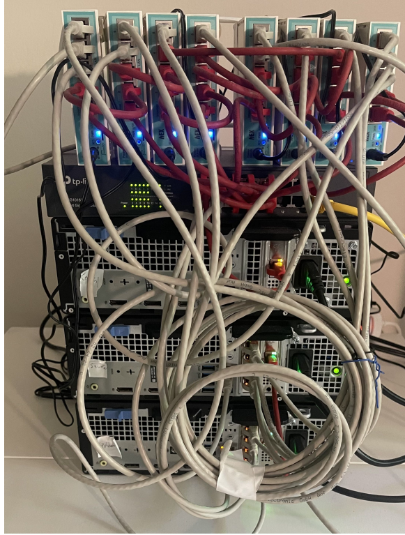
Figure 6.2.: Image of three computers, one switch and 8 routers.
